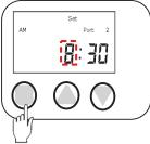
4. Press Up button "▲" or down button "▼" then set hour. Press Select button "•" and shift to "min" setting.
