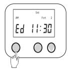
5. Enter end time and hold the Enter button "•" for 1 second to complete.
