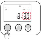
5. Press Up button "▲" or down button " ▼" then set min. Hold Select button "●" for 1 second to set time.
