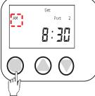
3. Press Up button "▲" or down button "▼" then select AM or PM. Press Select button "•" and shift to "hour" setting.
